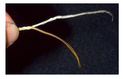
Form the loop as shown in Figure 6. Make sure you align the bundles as shown (same color over same color). Grasp the bundles at the bottom of the loop and twist the two bundles of same color together. Figure 6 shows white twisted onto white forming one large white bundle and yellow twisted onto yellow forming one large yellow bundle.
