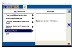
14. Click the parameter reset option and a reminder message will show that states that a parameter reset is required whenever an engine control module or the instrument cluster is replaced. The reset will erase keys stored in the cluster. Click the YES option. In some instances, the module replaced will be asked. Select PCM.
